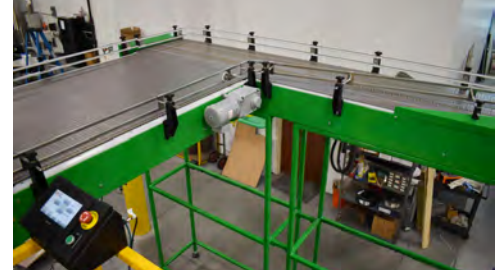
High Speed Single Filer with Mass Accumulation Table
