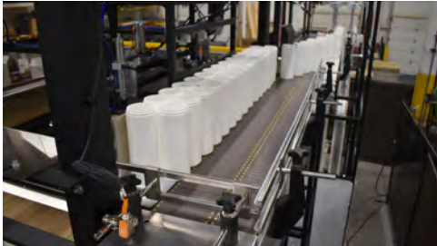
Dual Lane Discharge Conveyors
