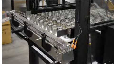
Single Lane Discharge Conveyors
