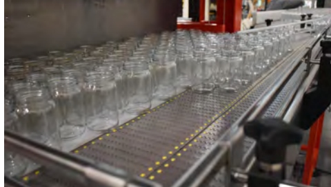
Dual Lane Discharge Conveyor
