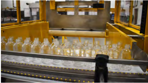
Single Lane Discharge Conveyor
